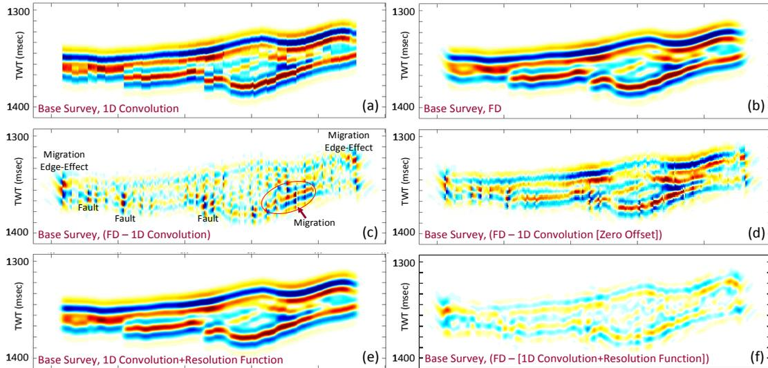
**Figure 3** (a) 1D convolutional modelling (b) FD modelling (c) FD – 1D convolutional modelling (d) FD (full offset) – 1D convolutional modelling (zero-offset) (e) 1D convolutional modelling + resolution function (f) FD – [1D convolutional modelling+resolution function]. To highlight the differences amplitudes are multiplied by a factor of 2 in figures (c), (d), and (f).
