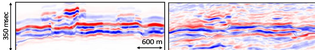
**Figure 1** Sim2Seis results (left) versus observed (right) seismic after PEM calibration.
