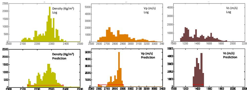
**Figure 2** Well log data (top) versus the predicted velocities and densities from the PEM (bottom).
