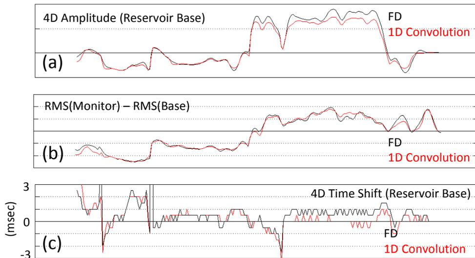
**Figure 4** 4D analysis of the seismic modelling. (a) 4D amplitude along the base of the reservoir. (b) 4D RMS amplitude. (c) 4D time shift at the base of the reservoir.
